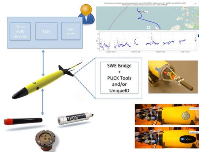
**Figure 3:** Interoperability standard solutions for sharing real-time data and instruments, here with optical and acoustic sensors installed on a commercial European glider (Sea Explorer, Alseamar), can deliver data and metadata in a harmonized communication and visualization framework (adapted from the NeXOS project for AtlantOS).
